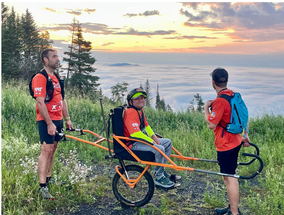
FIGURE 1 Joëlette set up, with one co-guide in the front and back of the wheelchair user.
