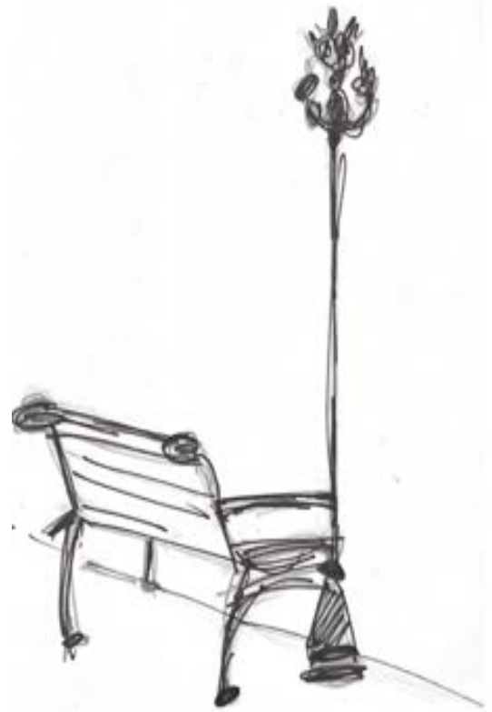
Figure 43. Lamppost as grab bar for the bench, by Lakoud.
